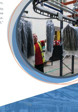
Bringing product up to the top mezzanine by conveyor from Goods In has massively simplified the delivery process and pushing the garments down the Slickrail line to the required location has increased our put-away speed.
