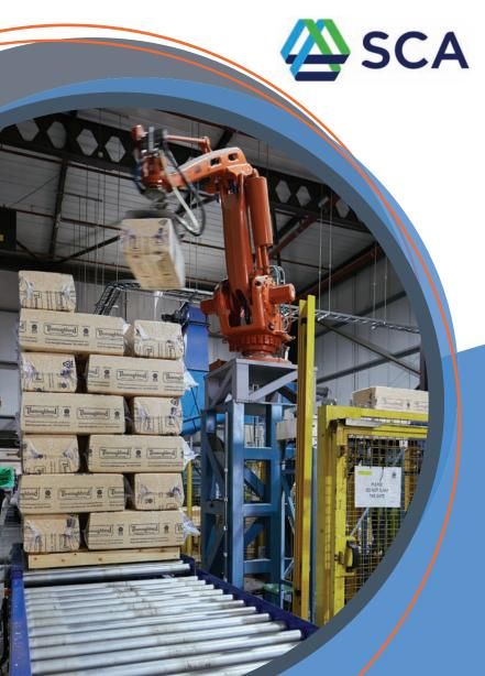
Leicester based, BS Handling Systems has installed an 18.5 metre long pallet roller conveyor for SCA Wood UK Ltd at its Melton facility. The pallet conveyor was installed as part of SCA Wood UK's plan to automate the palletisation of its softwood shavings bi-product.
