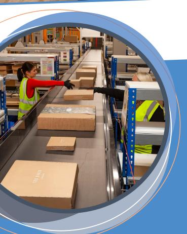
The ground floor conveyor has been installed at head height allowing for storage and walkways underneath. The system uses overhead scanners to read a licence plate number on the boxes and totes to divert them to the correct processing areas.
