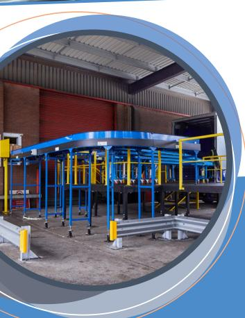
Waste cardboard packaging is placed onto the top tier of the conveyor. Each end of the top conveyor meets in the middle where waste cardboard drops onto a 24 metre long dunnage conveyor which transports it to a compactor. At this point, the two-tier conveyor system rises up to a height of 2.4 metres, allowing personnel and trucks to safely pass underneath.
